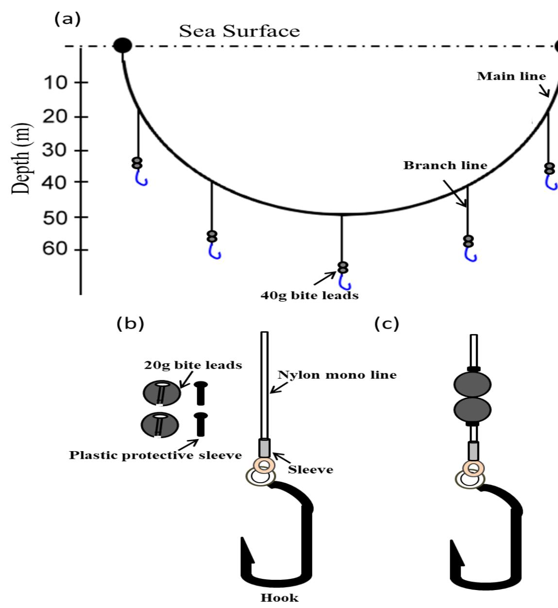
Fig. 6 (a) weighted branch lines (b, c)
